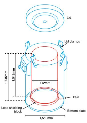
Figure 2: Dimensions of an example cylindrical flask
