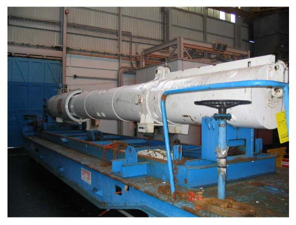
Figure 3: Control rod flask
