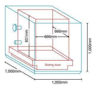
Figure 1: Dimensions of an example cuboid flask
