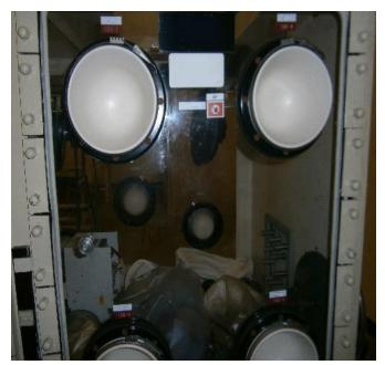
Above Left - Front of an older glovebox. Note the old gloves are 'posted' inside and blanking plugs fitted in their place.
