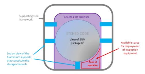
Any inspection solutions that require rotation of SNM packages should allow for lifting of the packages to avoid any damage that may be incurred by rotating the packages whilst in contact with the support structures. It should also be borne in mind that in some scenarios the packages are "co-joined".
