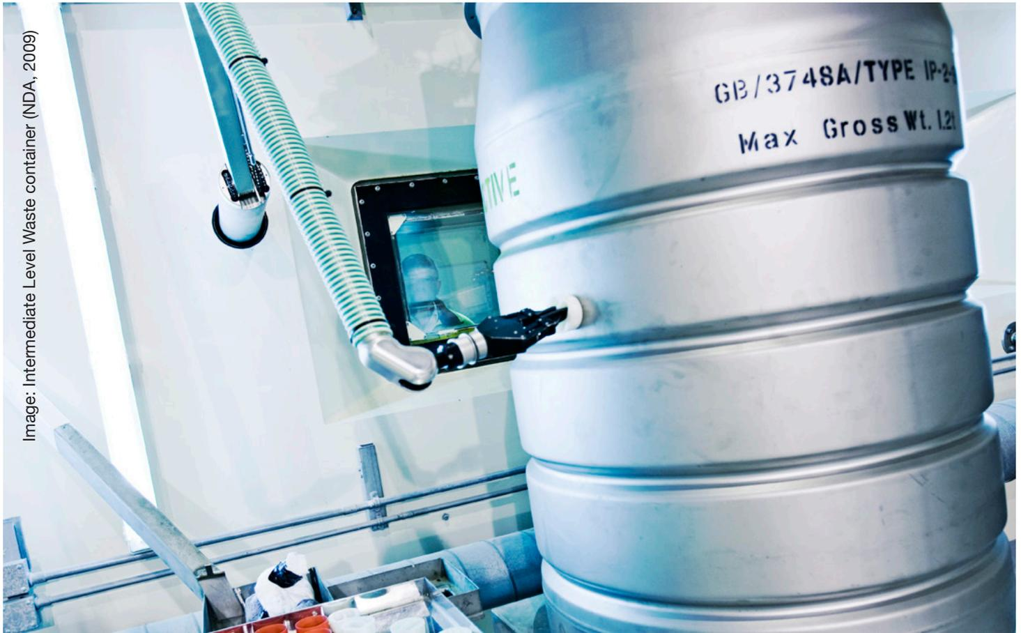
Image: Intermediate Level Waste container (NDA, 2009)
